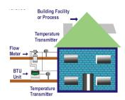
Net Heat Meters use accurately calibrated Ultrasonic Flow-meter, a matched pair of temperature sensors and computing unit inside the flow meter to calculate Net Heat consumed/transferred.
